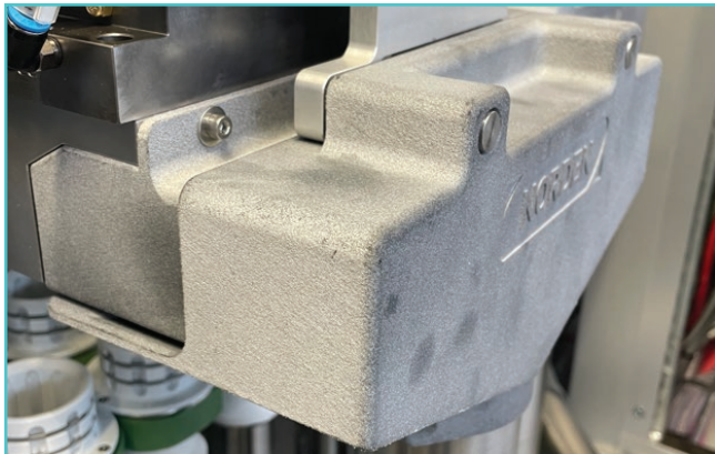
Trim waste chute before PostPro Vapor Smoothing
