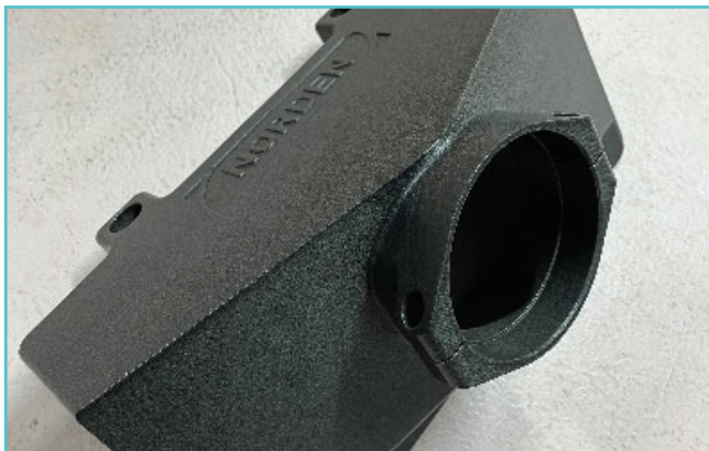
Trim waste chute after PostPro Vapor Smoothing
