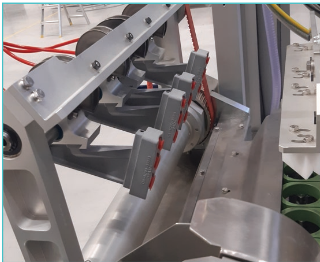
Pick & Place Format part before PostPro Vapor Smoothing
