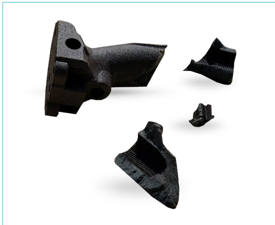
Raw part after impact test
