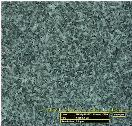
Figure 3. Un-processed SAF PA12 surface. x20 magnification
